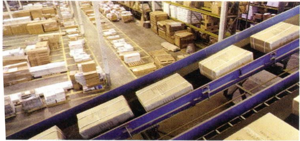
Photo 8.1 The coefficient of static friction between a package and the inclined conveyer belt must be sufficiently large to enable the package to be transported without slipping.
