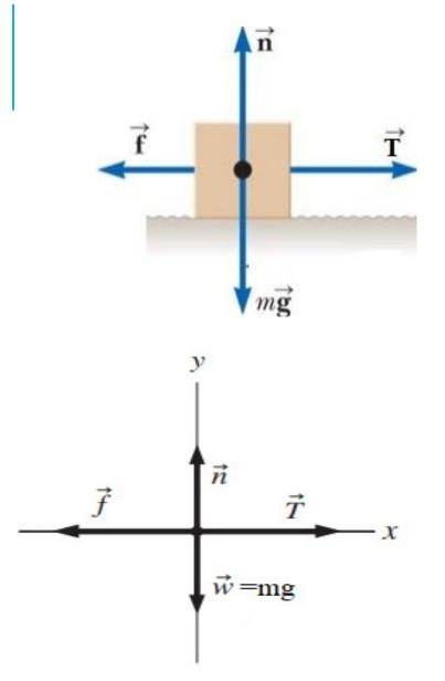
A free body diagram: is a force diagram that shows the relative magnitude and direction of all forces that acts on an object in a specific situation
