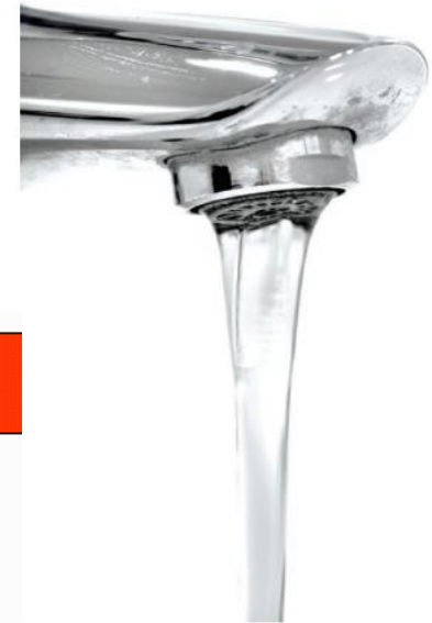
Figure 9.23 Demonstrating the continuity equation at a bathroom sink. Notice that the stream of water is narrower here the flow speed is faster. Michael Bodmann/Getty Images
